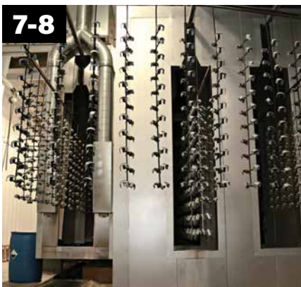
7-8 A 200 MPH air blast removes water drops from the pre-treated aluminum. A convection oven completes the dry-off process.
